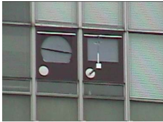
Figure 7: Driving-rain gauges in the west facade of the Main Building at position P5 (left, d.r. gauge II with wiper) and P4 (right, d.r. gauge I without wiper).
