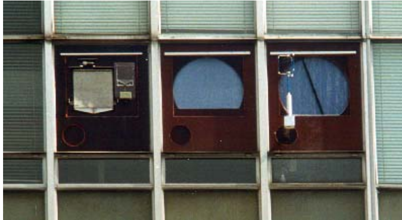
Figure 3.8: The four driving rain gauges on the west façade of the Main Building during the third measurement period from 16 September 1998 to 25 February 1999. From left to right: DTU (position P7), CTH (P7), TUE-I (P5) and TUE-II (P4). The ultrasonic anemometer has been mounted near TUE-II. Photograph by Ben Elfrink.
