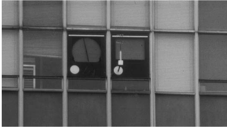
Figure 3.7: The two driving rain gauges on the west façade of the Main Building during the first measurement period from 11 December 1997 to 7 July 1998. From left to right: TUE-II (position P5) and TUE-I (P4). The ultrasonic anemometer has been mounted below TUE-I. Photograph by Ben Elfrink.
